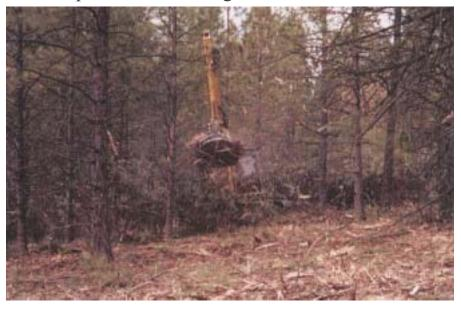
Slashbusting<sup>®</sup> is a very cost effective way to construct firebreaks or fire lines as shown in these side by side tables.
