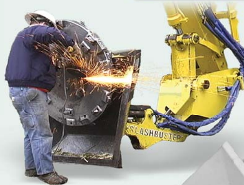
Sharpening "S-7" teeth in the field with an angle grinder
