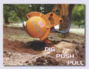
Use the **Double Heel Rack** to remove obstructions and dig around the stump when grinding below soil level
