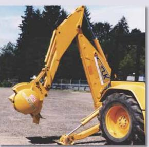
Mounts on any backhoe with at least 80 horsepower
